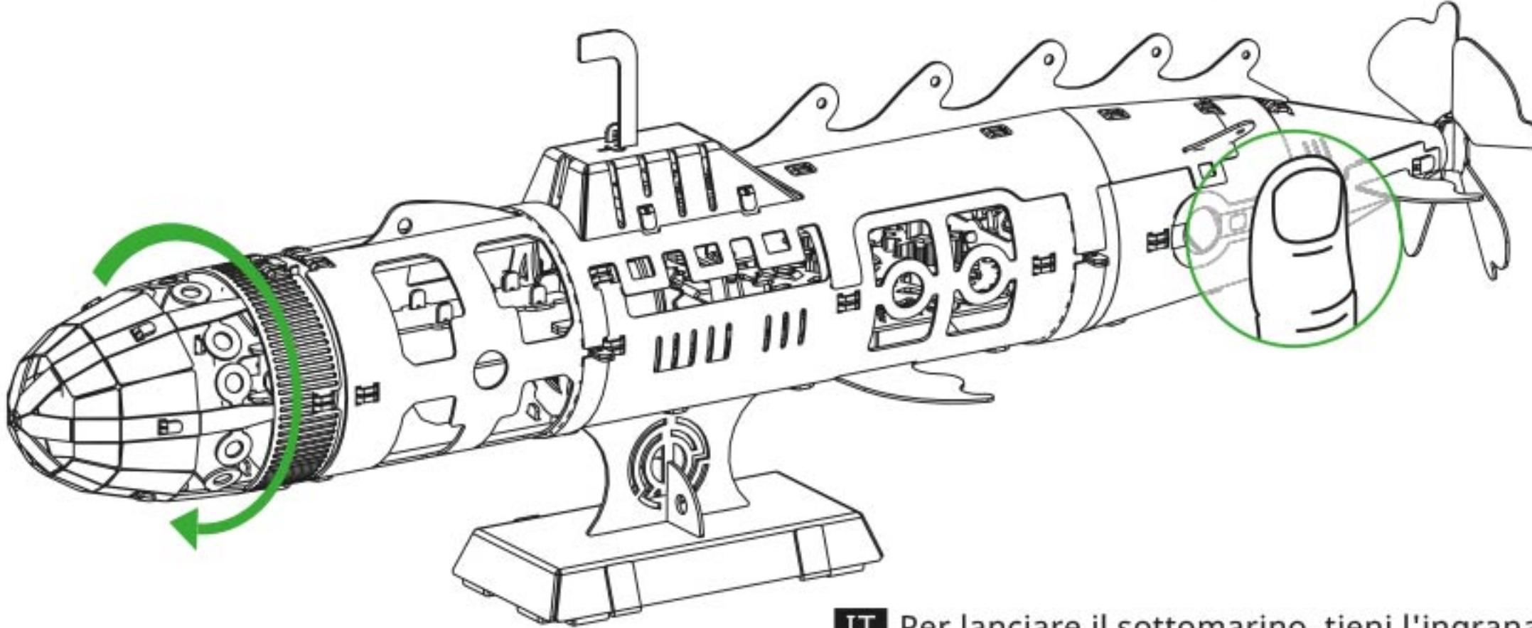
**EN** To launch the sub, hold rear gear with your finger and turn the bow clockwise, then release the gear.
