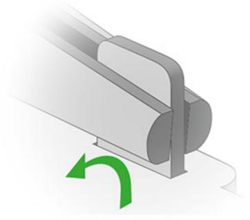
Use pliers to bend the fasteners
