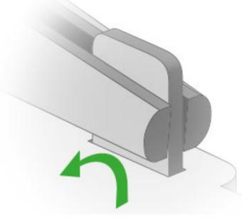
Use pliers to bend the fasteners
