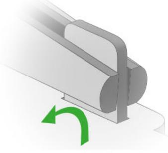
Use pliers to bend the fasteners
