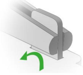
Use pliers to bend the fasteners
